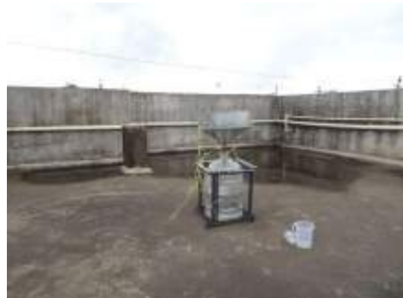
Fig. 4.6: Rainwater sampling apparatus kept in open to avoid any kind of interference
