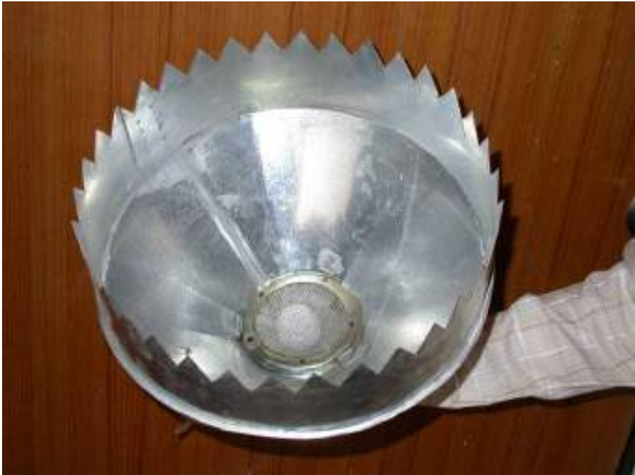
Figure 2. A circular wire-mesh disk and the plastic ball placed inside the funnel.
