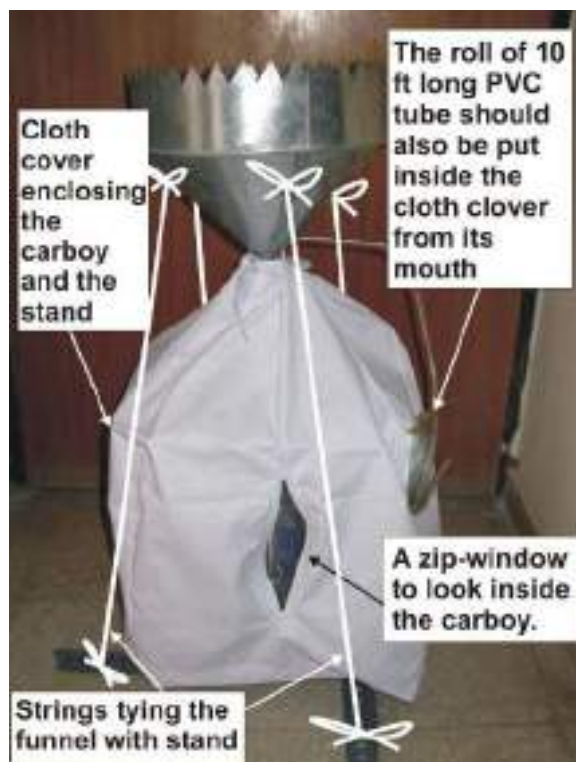
Figure 5 A cloth cover enclosing the rainwater sampling device.
