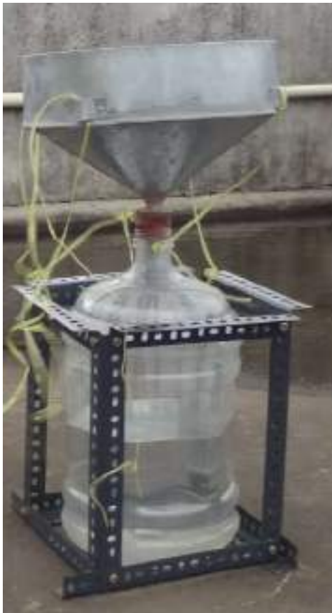
Fig. 4.5: Arrangements for prevention of evaporation loss from the rainwater sampling apparatus
