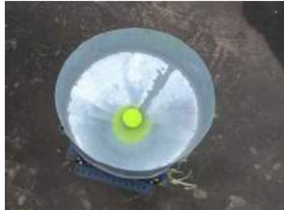
Fig. 4.5: Arrangements for prevention of evaporation loss from the rainwater sampling apparatus
